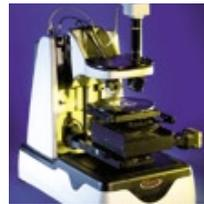
Surface roughness metrology systems include Stylus Profilers and Optical Profilers.
