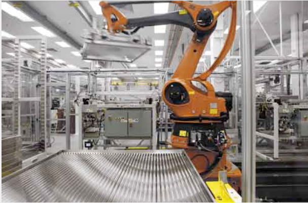
▲ Solyndra's fully-automated production line uses robots to move cylindrical substrates into a mounting.
